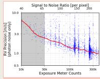
Photon-limited single measurement precision as a function of exposure meter setting and signal-to-noise ratio. The red line traces the lower 30th percentile of the individual measurements (blue points). Signal-tonoise ratios below 70 (gray shading) are not officially supported by the pipeline and may produce erratic
