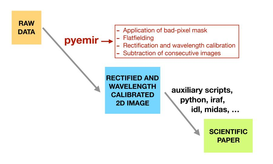
The Python package **pyemir** helps to generate a rectified and wavelength calibrated 2D image. From this point, the astronomer can use its favourite software to proceed with the spectra extraction and analysis.
