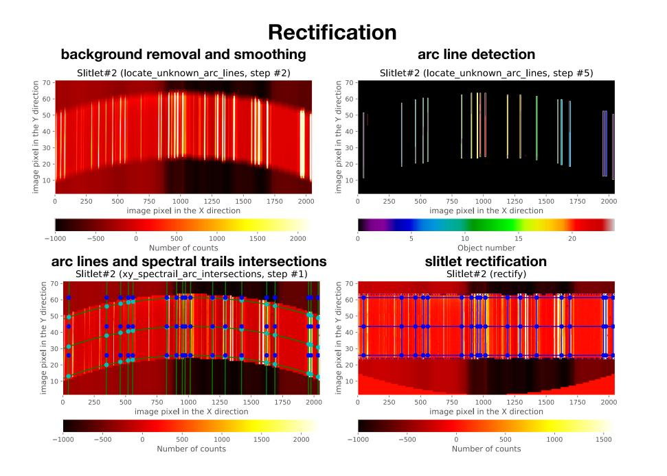
Once the slitlet boundaries have been determined, it is possible to rectify each 2D slitlet. In this example, an arc exposure is being analysed in order to determine the intersections between arc lines and spectral trails. These reference points allows the computation of the rectification transformation.
