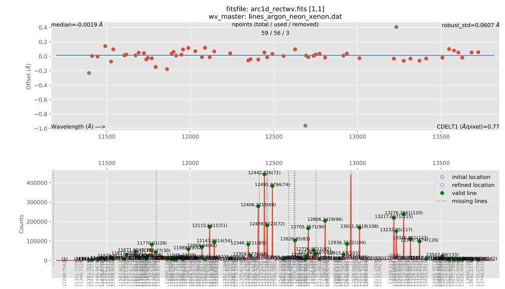
The preliminary wavelength calibration is then improved by using additional (faint) arc lines, in order to achieve a typical r.m.s. of the order of 1/10 pixel.
