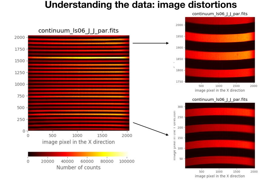
The raw EMIR 2D spectroscopic images exhibit geometric distortions. This effect is clearly noticeable in this sample continuum exposure, where only evennumbered slitlets are opened (the odd-numbered slitlets where closed).
