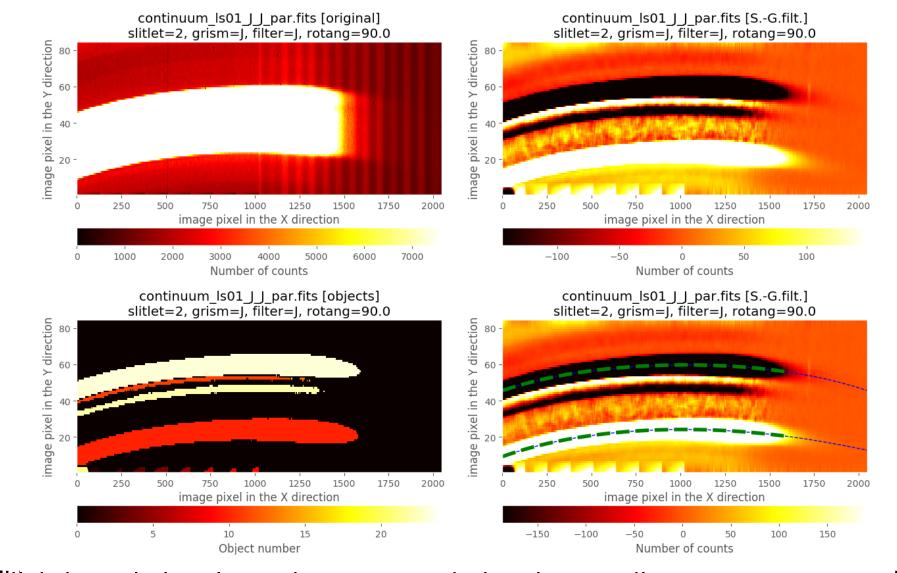
Slitlet boundaries have been computed using continuum exposures with alternate even- and odd-numbered slitlets opened and closed. After smoothing the image to facilitate the task, the boundaries are determined using the first derivative of the signal when moving in the vertical (spatial) direction.
